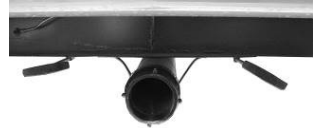
Black/Grey Tank Drain and Valves
